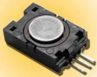
Figure 6: Infusion pump force load cell
